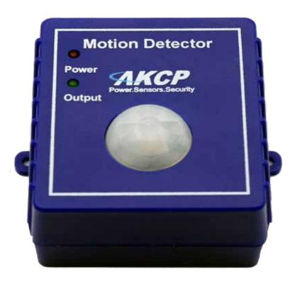
Infrared motion detection, is a hardware based motion detection technology that will detect movement up to 3 meters away. MD00 can be daisychained together with a maximum of 10 in a single string, meaning a single sensor port can support 10 motion sensors. When one motion sensor in the string is in critical state the whole string will show as critical.
