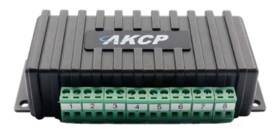
The IO-digital8 sensor adds 8 dry contacts to the securityProbe or expansion module base unit. With 8 ALARM/NORMAL indication in the securityProbe 5E web interface it provides instant notification for changes of status. The sensor can be mounted on a wall by your alarm panel, or using our DIN rail clips can be DIN rail mounted. A standard CAT5 cable connects the IO-digital8 sensor to the intelligent sensor port.
