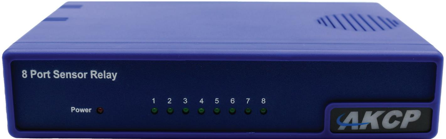
The 8 Port Sensor Relay is specially designed multi-port relay for advanced process control. The 8 Port Sensor Relay is easily controlled by any of AKCP's extensive selection of sensors. The relay can provide automatic responses to sensor status changes. Setting up the sensor controlled relay is easy with its built in autosense feature and user friendly web interface.
