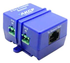
The single port RJ-45 Dry Contact Sensor with an ALARM/NORMAL indication in the software. Can have up two on a SP2, four on an SP2+ eight on a SP8 and 600 Dry Contact Sensors on a securityProbe unit. Dry contact sensors are user definable and can be used to detect many different inputs such as UPS status, security systems, air conditioning status.
