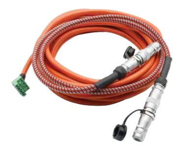
The AKCP ropeFuel sensor is a rope-type leak detector that connects to any AKCP sensorProbe or securityProbe RJ-45 Intelligent Sensor Ports and facilitates the detection of fuel and other liquids. The AKPP rope Fuel sensor provides distributed leak detection for a wide range of applications such as monitoring for fuel leaks beneath or around backup generator fuel tanks, fuel storage areas, or fuel transfer stations.
